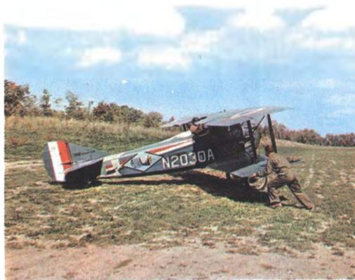
Steering the plane on the ground requires a helping hand; one wing must be held steadfast for the turn.
